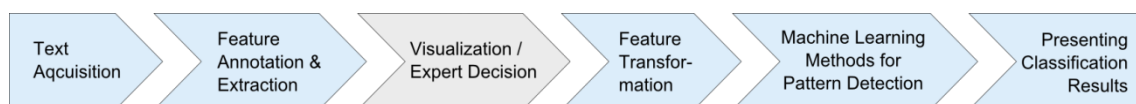
Figure 1-1: A processing pipeline concept that contain various feature preparation steps and machine learning methods in order to perform a text classification.
