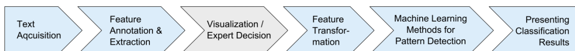
Figure 1-1: A processing pipeline concept combining feature preparation steps and machine learning methods in order to perform a text classification.
