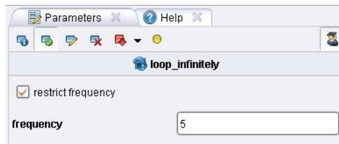
Figure 5.9: The parameter tab with restrict frequency checked: The conditioned parameter is shown
